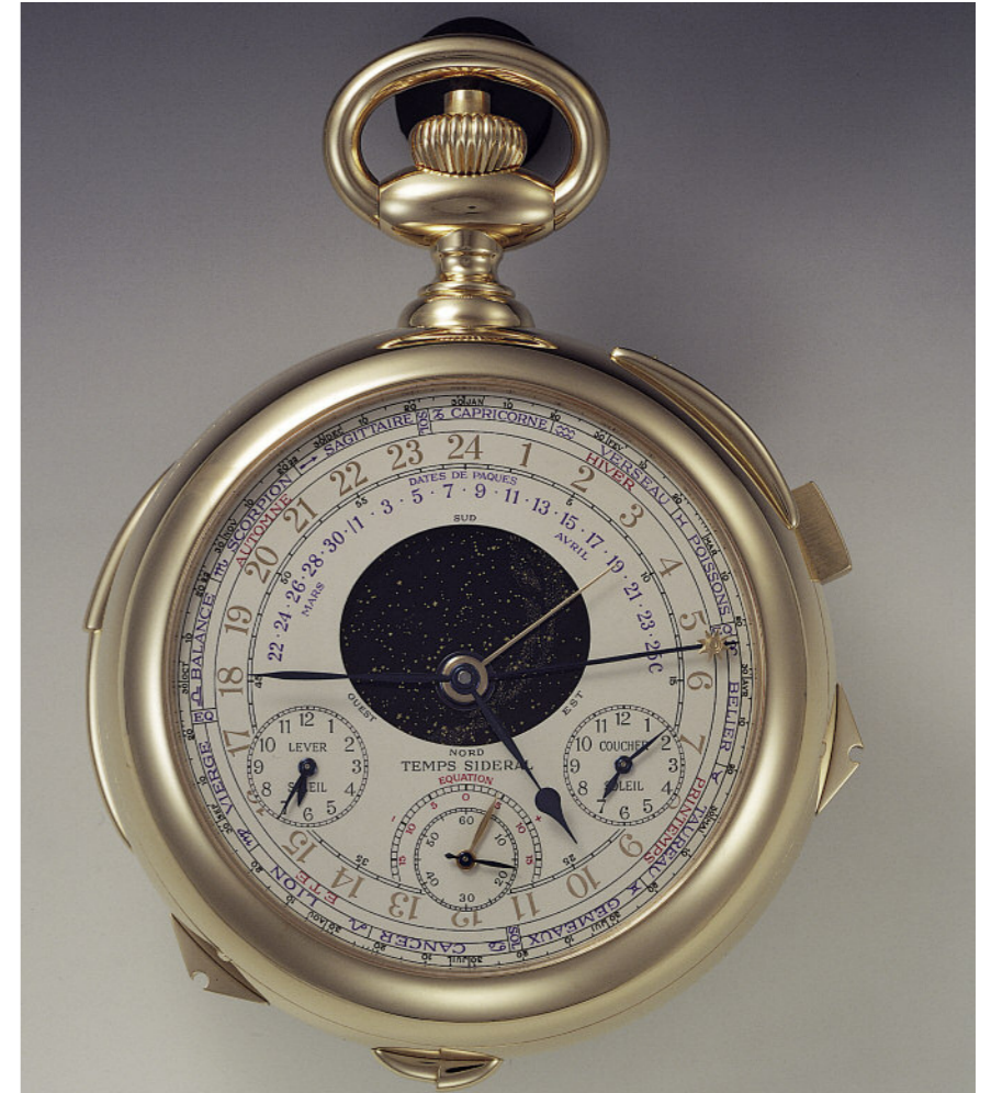
Above: Back dial of Caliber 89 with the sky above Geneva; the dial indicates solar time, equation of time, sunrise and sunset, date of Easter, and signs of the zodiac. Bottom left: Caliber 89 in its presentation case. Below: The workbench of master watchmaker Paul Buclin, who worked on Caliber 89 for many years.
